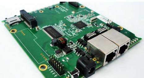
WPJ531 is a reliable and dynamic wireless embedded board based on the Atheros AR9531 CPU. It features a 550MHz network processor and integrates a 2.4Ghz 2x2 internal on-board radio and 1 miniPCle slot that supports 802.11n radio. Embedded with 64MB memory and 8MB Flash, WPJ531 provides the ideal platform for any applications. WPJ531 has integrated Power over Ethernet (PoE) features that allows WPJ531 to be used in areas where power outlets are not readily available.
