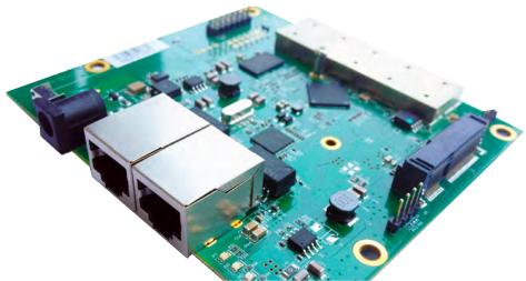
WPJ342 is a capable and reliable wireless embedded board based on the Qualcomm Atheros AR9342 CPU. It features a 560MHz network processor and integrates a 2x2 internal on-board radio and 1 miniPCle slot that supports 802.11n radio. Embedded with 64MB memory and 16MB Flash, WPJ342 provides the ideal platform for any applications. WPJ342 has integrated Power over Ethernet (PoE) features that allows WPJ342 to be used in areas where power outlets are not readily available.
